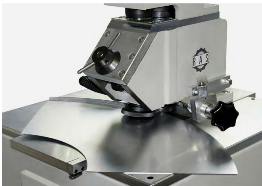
Automatic sheet guide system
