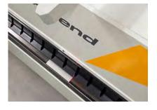
The ViN uses a laser beam to show the exact side loading position of the part.
