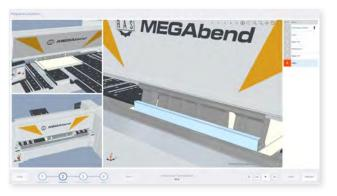
A 3D simulation shows the bending sequence, the tool setup and the loading position of the part.
