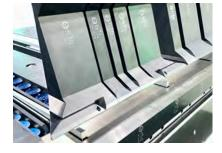
SnapTools with a hinged foot automatically move out from parts with side flanges.
