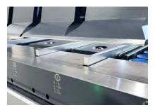
The stop fingers are able to move as close as 20 mm to the bending line and thus can position even very narrow parts.
