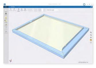
The Bendex software imports a step file of the part and automatically programs the bending sequence.
