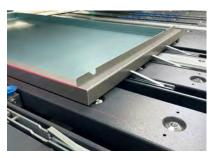
Suction bars next to the stop units hold the part for subsequent bends to the stop fingers.
